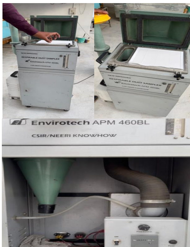
Fig3. 1 Respirable dust samplers
